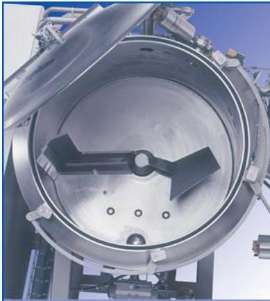
Vessel with mixing arm and steam nozzles
